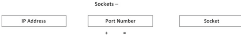
Figure 3-2. A socket consisting of IP address and port number
